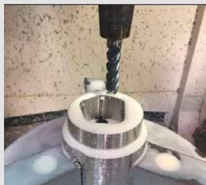
Walter special tool: New chip breaker design creates short chips which make chip evacuation easier.
